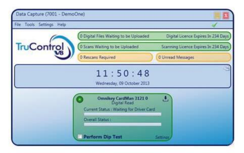
To download a driver's card, insert the driver's card into the reader (chip facing away from you), the application will then display the progress of the read in the card reader window (usually identified as Omnikey CardMan). The read processes takes approximately 30 secs to 1 min.
